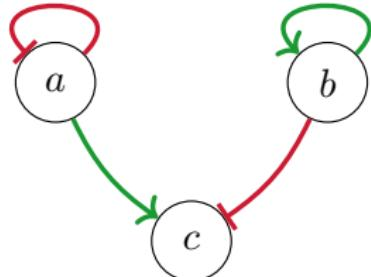
$$\begin{aligned}f_a(\mathbf{x}) &= \neg x_a \\f_b(\mathbf{x}) &= x_b \\f_c(\mathbf{x}) &= x_a \wedge \neg x_b \quad x_a \vee \neg x_b\end{aligned}$$
